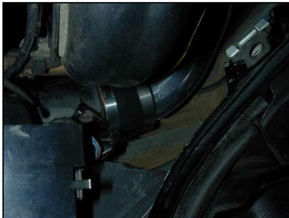
Photo 6.5. Intake Pipe installed on MAF.
