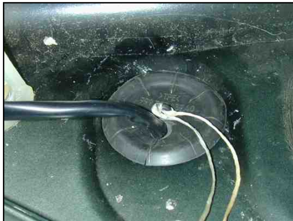
Photo 11.7. Harness inserted through modified plug cap.
