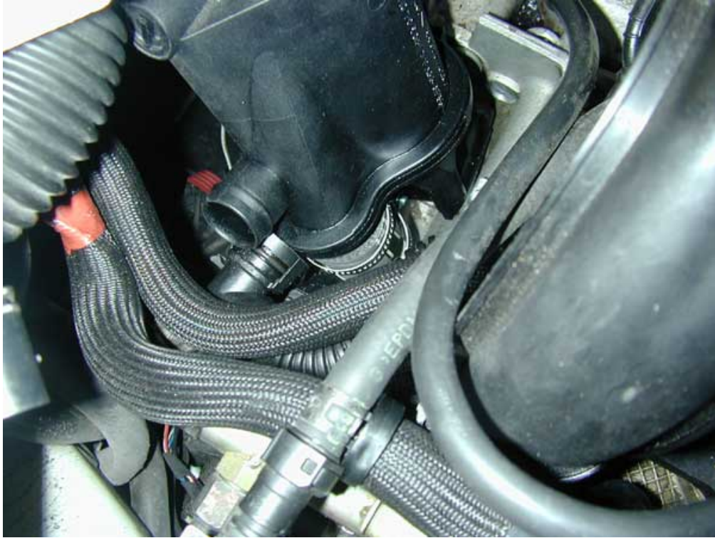
Photo 9.5. Air-oil separator during installation.
