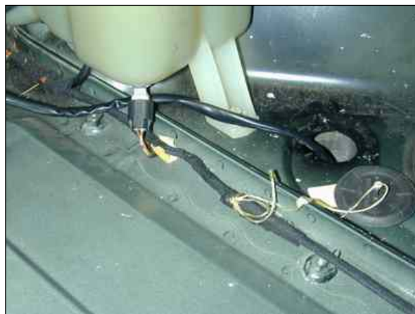
Photo 11.5. Harness dropped through trunk hole.
