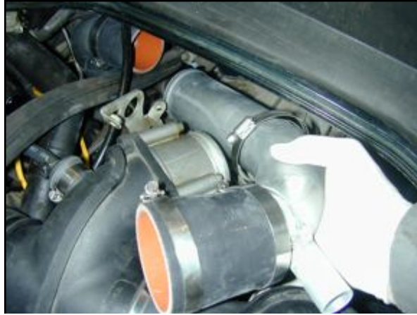
Photo 14.4. Boostpipe #3 ready to install.
