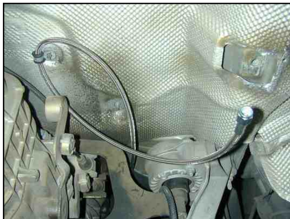
Photo 10.1. -4AN Oil Line looped through clamp.
