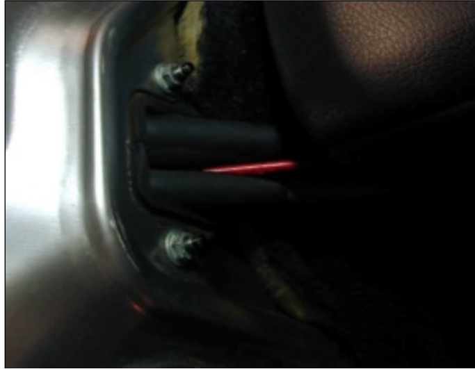
Photo 19.1. Boost Gauge vacuum line routing through firewall grommet.
