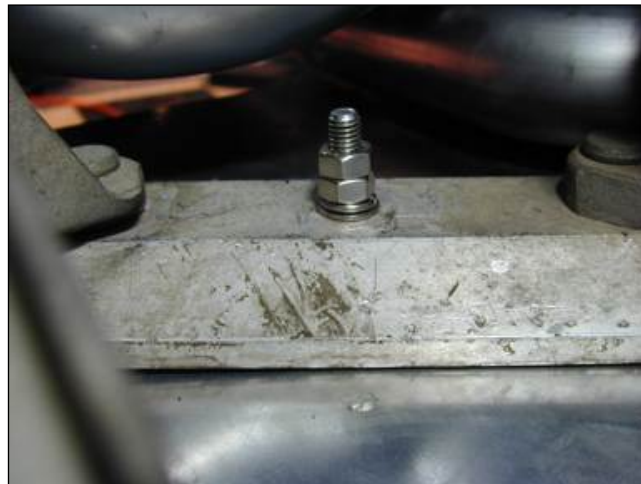
Photo 17.5. Intercooler Heatshield center fastener installed.
