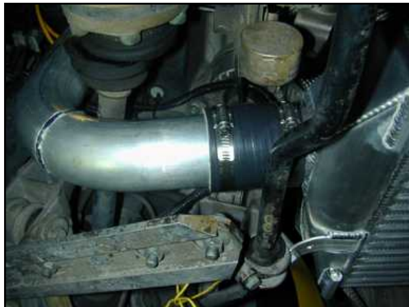
Photo 14.3. Boostpipe #2 bottom installed.
