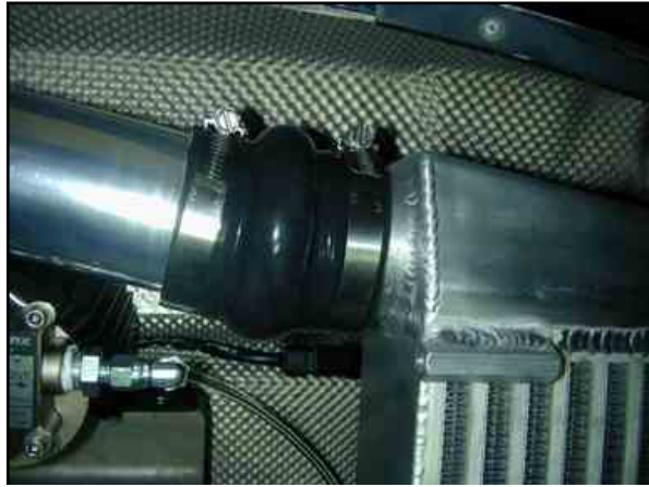
Photo 13.1. Boostpipe #1 hump hose installed.
