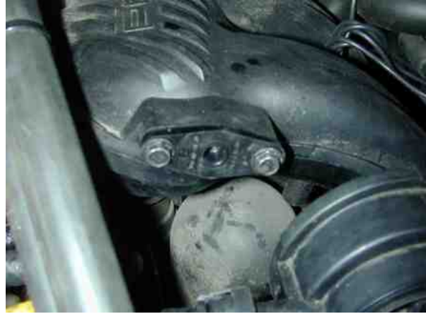
Photo 1.4. Plenum port cover plate.
