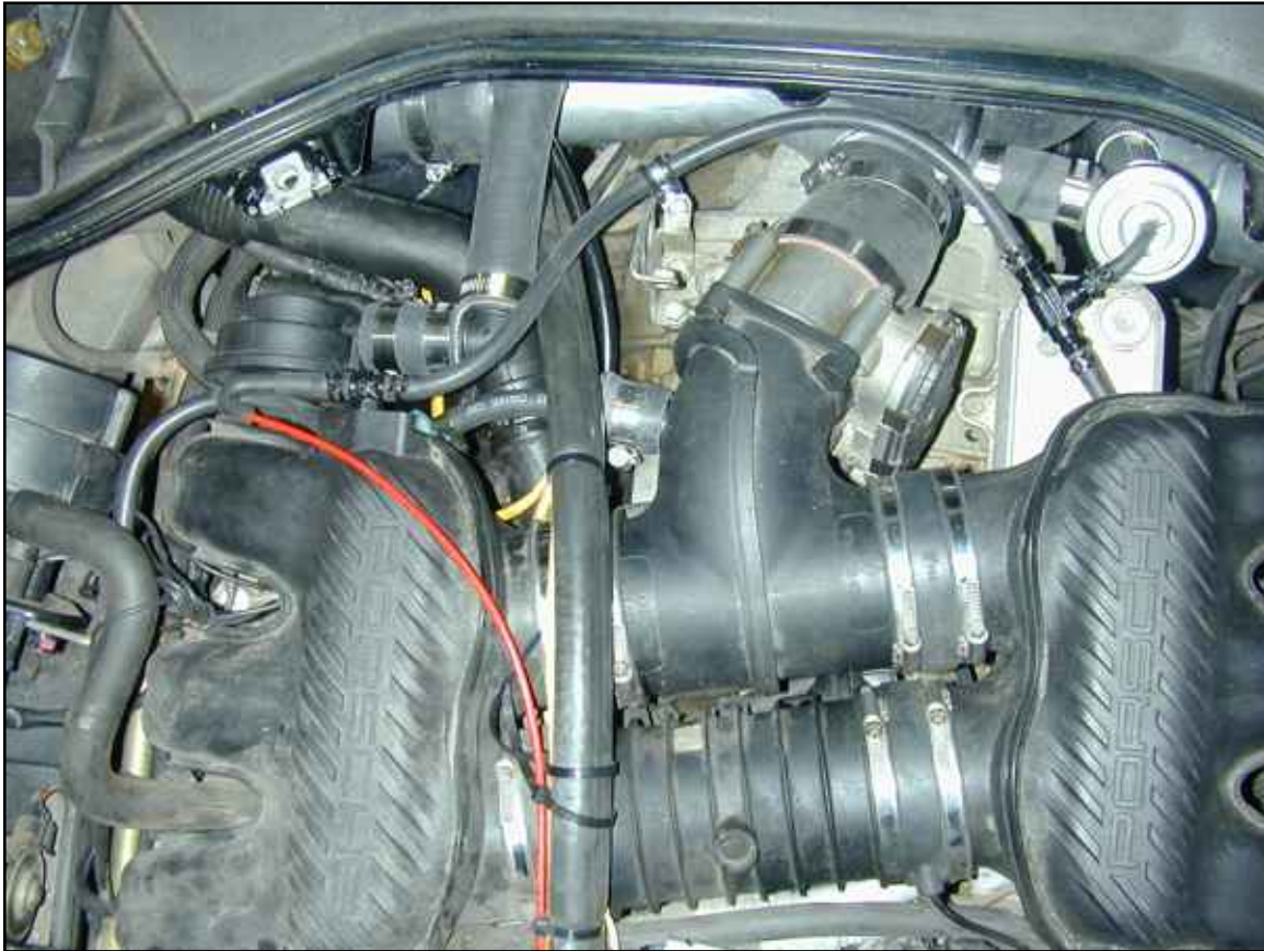
Photo 16.0. Vacuum-Boost Hose installed (top view).
