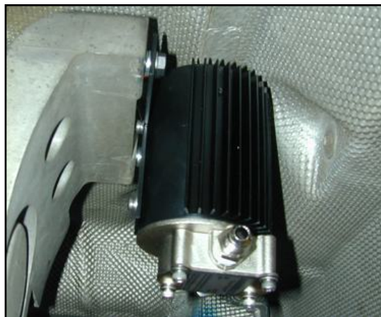
Photo 10.0. Scavenge Pump mounted.
