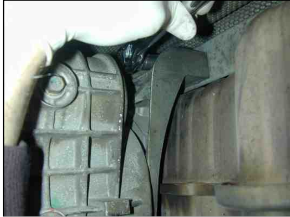
Photo 5.4. Ratchet on muffler support bolt.
