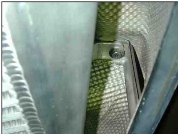
Photo 12.1. Intercooler rear support bolt.
