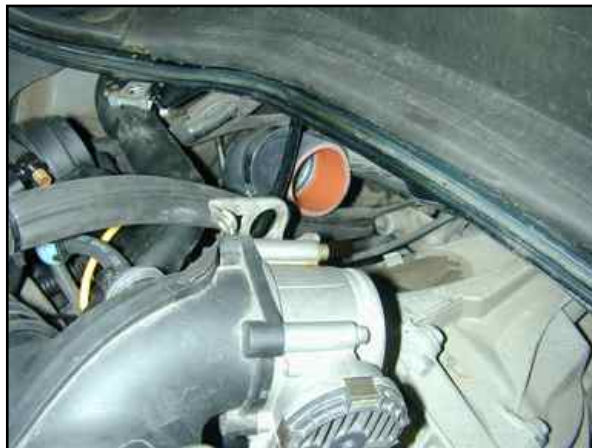
Photo 14.0. Top of Boostpipe #2 in position.
