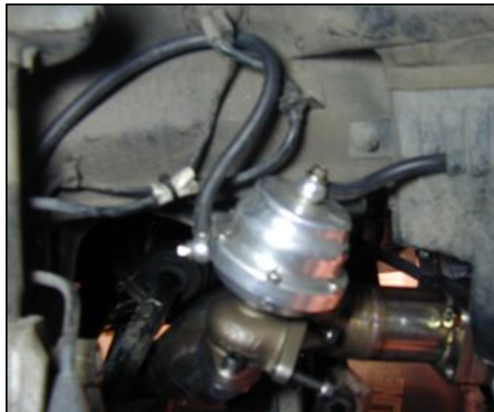
Photo 16.4. Wastegate mounted with hoses attached.
