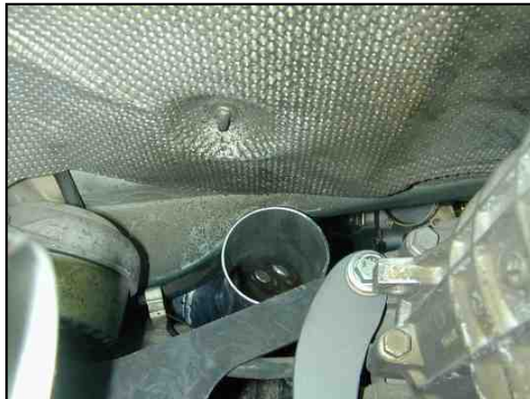
Photo 6.7 Rear view of Intake Pipe.
