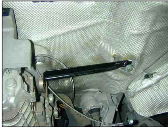
Photo 10.2. Intercooler Bracket mounted.
