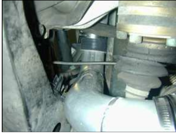
Photo 14.1. Boostpipe #2 Line clearance from -4AN Oil Return Line.
