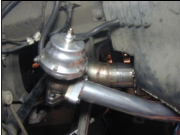
Photo 16.5. Wastegate Pipe installed.
