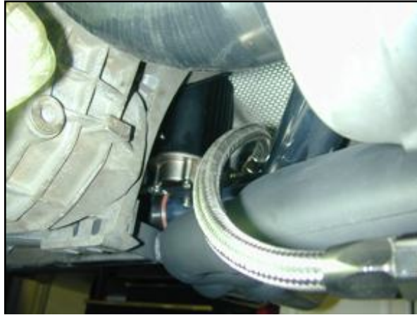
Photo 13.7. -6AN Turbo Oil Drain Hose clearance.
