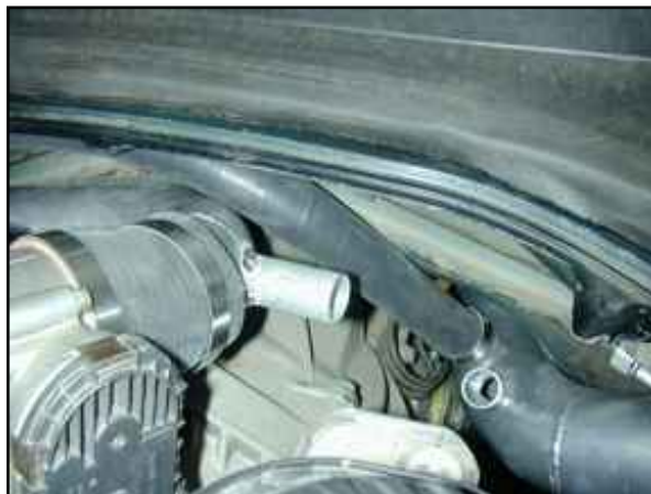
Photo 15.0. Crankcase Hose connected to bottom port of Intake Pipe.
