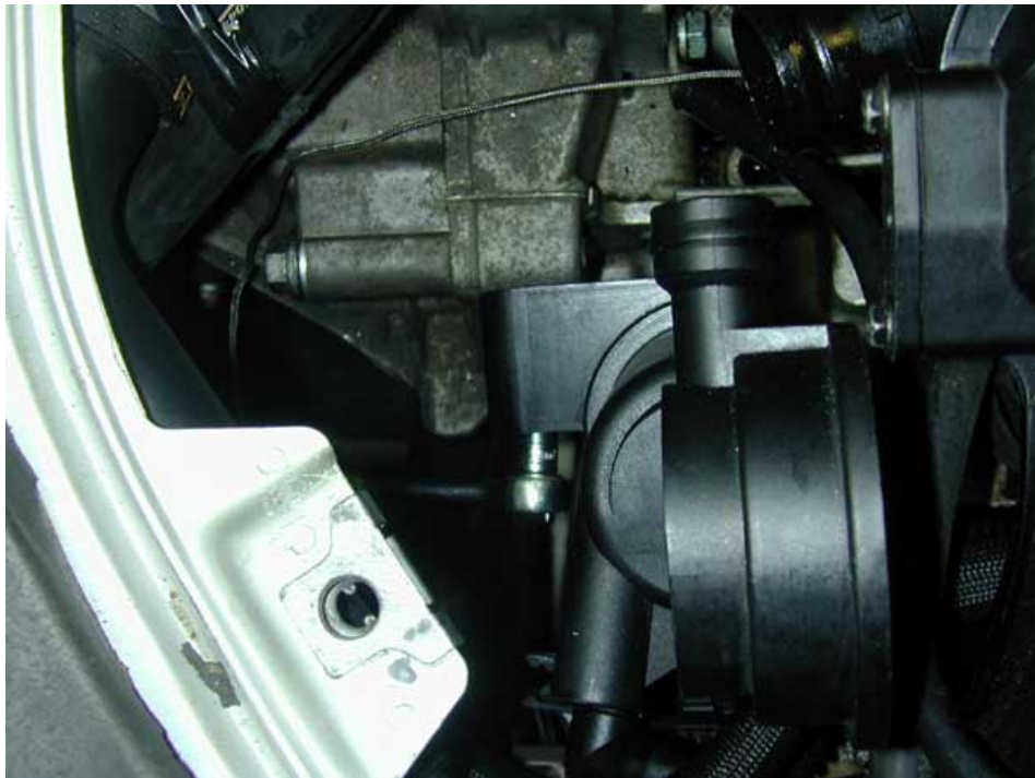
Photo 9.2. Removing 10mm bolts from air-oil separator.
