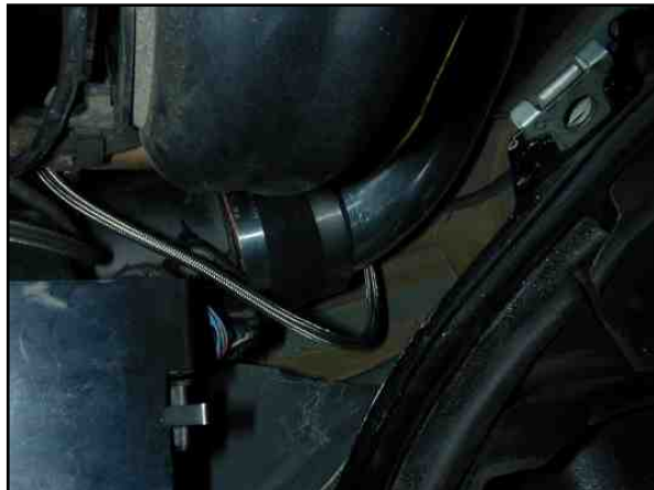
Photo 8.1. -3AN Oil Line routing.
