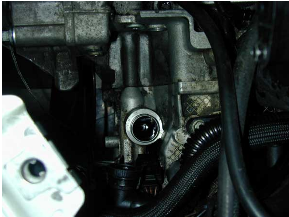
Photo 9.3. Air-oil separator removed.
