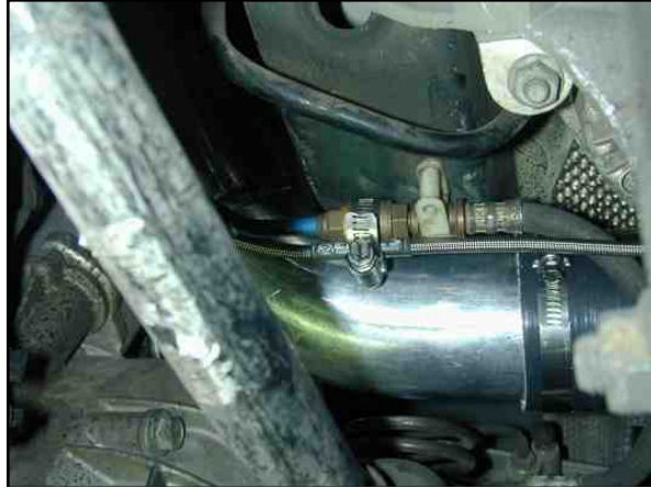
Photo 8.2. -3AN Oil line secured.
