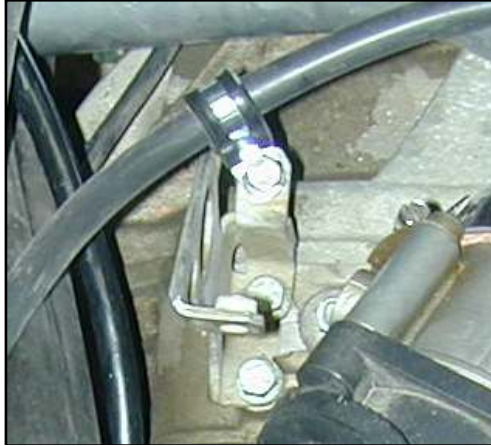
Photo 16.1. Vacuum-Boost Hose clamp eye bracket location.
