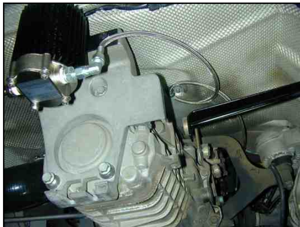
Photo 10.3. -4AN Oil Line installed.
