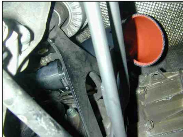
Photo 6.9. 45 degree silicone installed.
