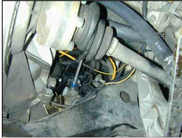
Photo 9.7. Oil Return Assembly installed.
