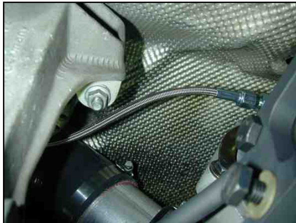
Photo 8.3. -3AN Oil line connected to turbo.
