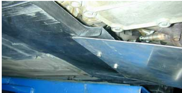
Photo 17.3. Intercooler Heatshield front fasteners installed.
