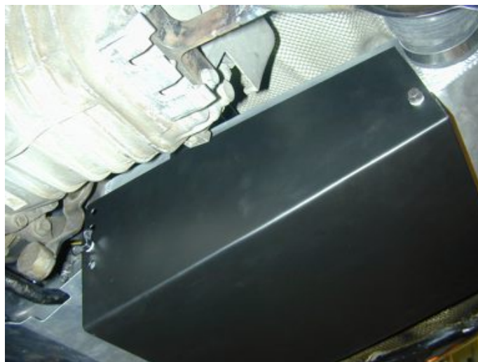
Photo 18.2. Intercooler Air-duct installed.
