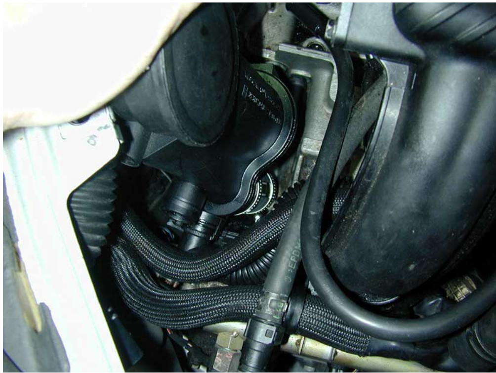
Photo 9.6. Air-oil separator with small vent lined up for insertion.
