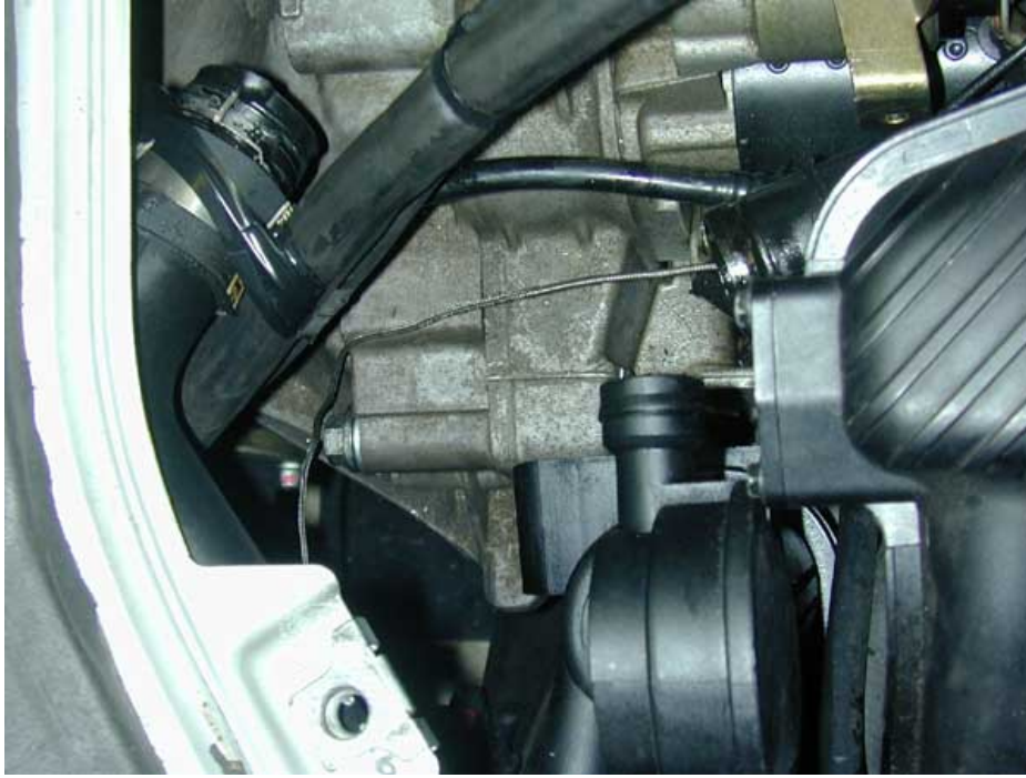
Photo 9.0. Temporarily securing plastic oil filler tube.
