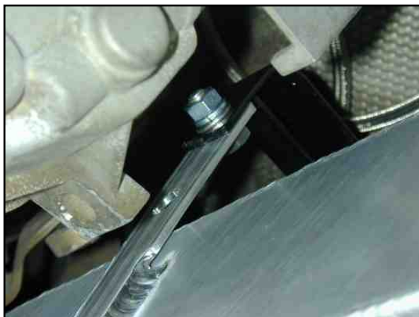
Photo 12.2. Intercooler top support fastener.
