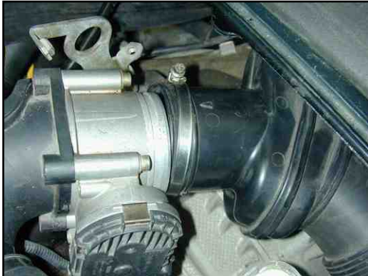
Photos 3.0-3.1. Intake clamps loosened.
