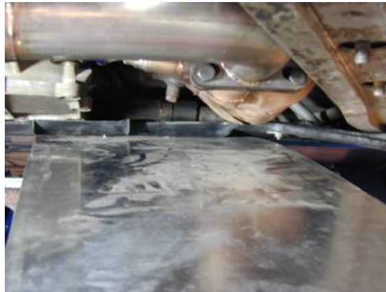
Photo 17.1. Intercooler Heatshield attached to plastic undertray.
