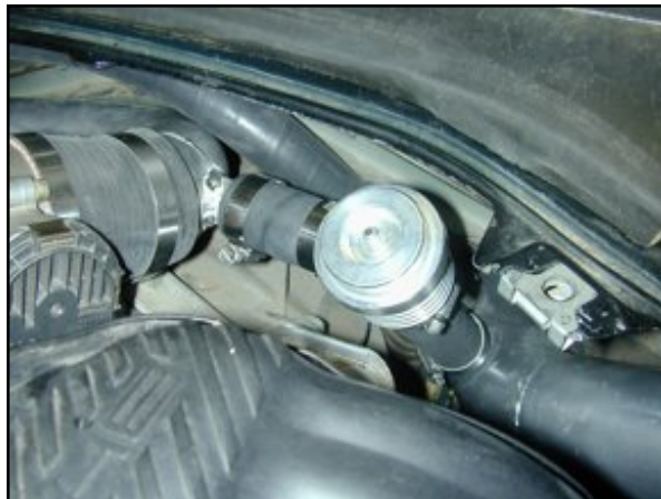
Photo 15.3. Recirculation Valve Assembly installed.
