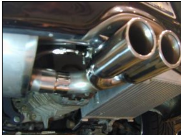
Photo 13.5. Muffler mated to tip.
