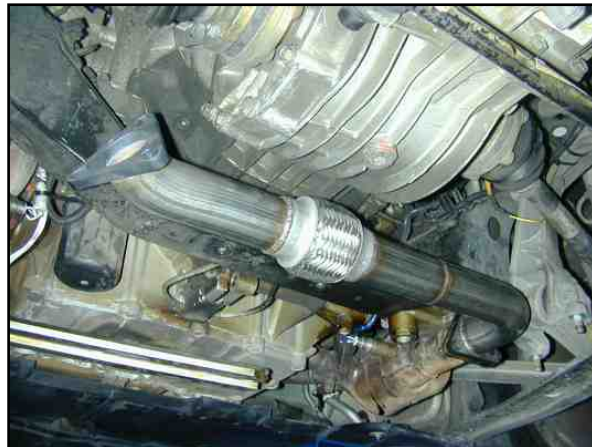
Photo 7.2. Right side exhaust pipe installed.
