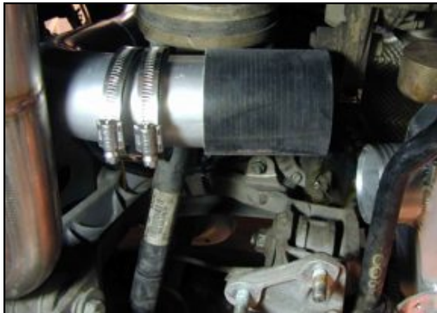
Photo 14.2. Bottom of Boostpipe#2
