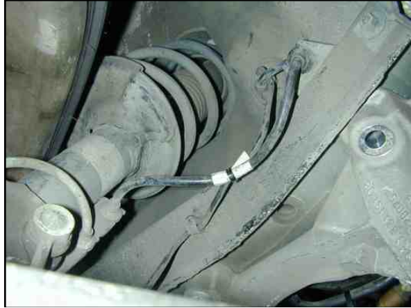
Photo 7.3. ABS cable secured with tie-wrap.
