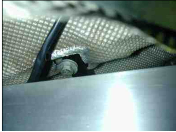
Photo 12.3. Intercooler Bracket bolt.
