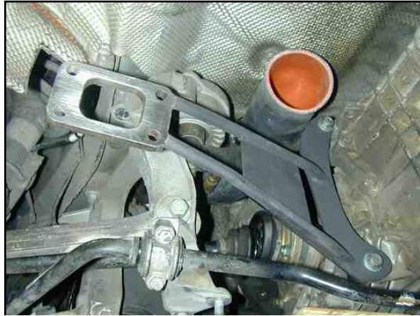
Photo 7.1. Turbo Bracket installed.
