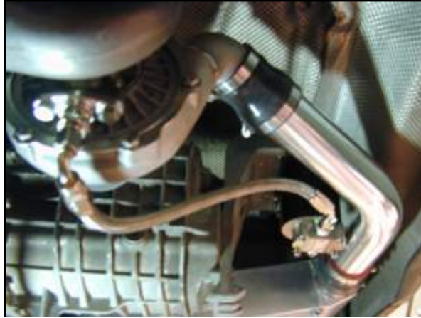
Photo 13.3. -6AN Turbo Oil Drain Hose installed.
