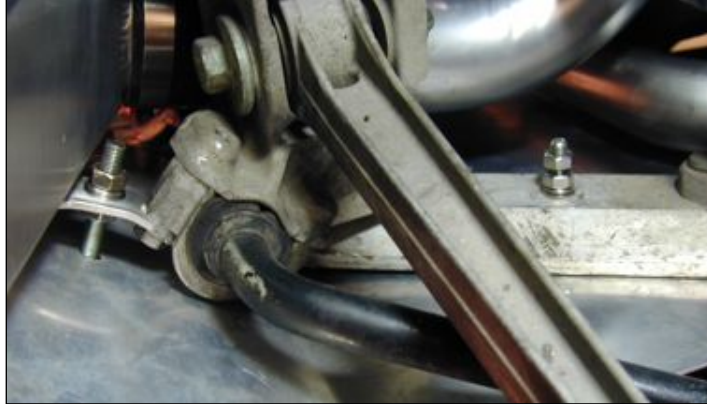
Photo 17.6. Intercooler Heatshield rear and center mounts.
