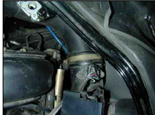
Photos 3.0-3.1. Intake clamps loosened.
