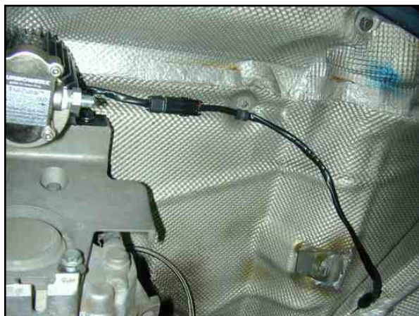
Photo 11.10. Harness connected to Scavenge Pump.
