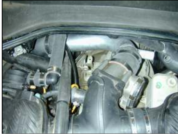
Photo 15.1. Crankcase Hose installed.
